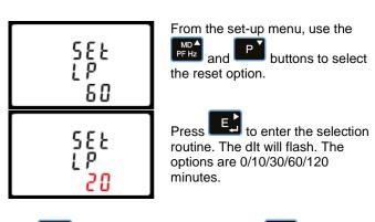
Press to confirm the setting and press to return to the main set up menu.
