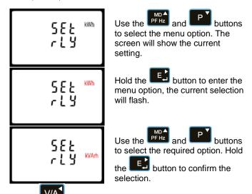
Hold the button for 3 seconds to exit the set up menu.
