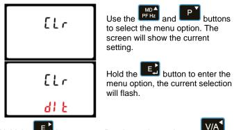
Hold the button to confirm the setting and press to return to the main set up menu.
