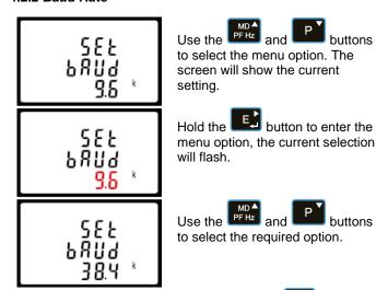
On completion of the entry procedure, hold the button to confirm the setting.
