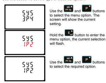
Hold the button to confirm your adjustment. Hold the button for 3 seconds to exit the set up menu.
