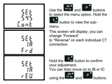
Hold the button for 3 seconds to exit the set up menu.
