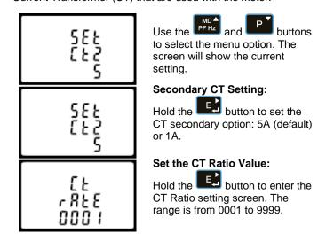
The CT Ratio is the CT Primary divided by the CT Secondary. For Example: 200/5A Current Transformers - 200÷5=40, so the CT Rate would be 0040 and the CT2 would be 5.
