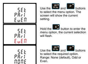
On completion of the entry procedure, hold the seconds until the selection stops flashing.
