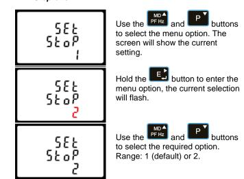
On completion of the entry procedure, hold the button for 3 seconds until the selection stops flashing.
