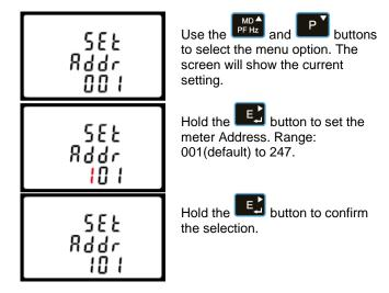
Use the buttons to choose the necessary number, then press the button to move along to the next number. To save the new setting, hold the button seconds until the selection stops flashing.
